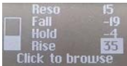
Macro Assign display for setting modulation amounts
