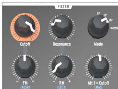
The Filter section
