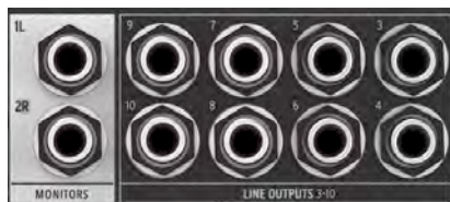
Rear panel audio outputs, with Speaker outputs at left
