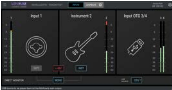
The Inputs tab in macOS, with metering and controls for the two Inputs and the OTG port
