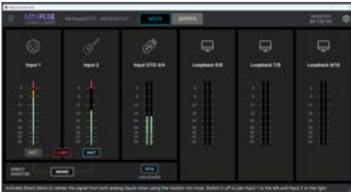
The Inputs tab in Windows, with metering for physical, OTG, and the Loopback inputs which are then sent to their associated outputs (as explained in the Loopback Recording chapter).
