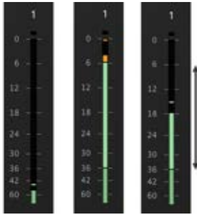
Level settings. L to R: too low, too high (distorted), and ideal
