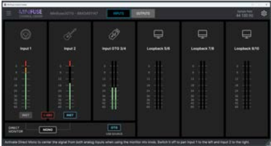
The Inputs tab, with metering for physical and Loopback inputs
